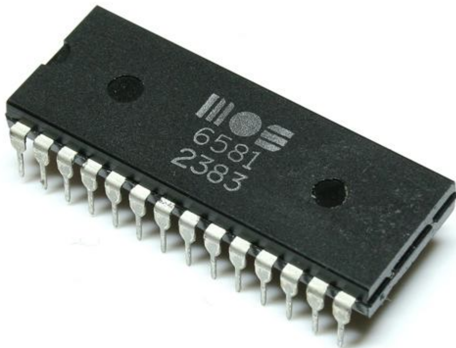
Figure 1. Sound Interface Device (SID), MOS Technology, 1981. (Photo courtesy Chris Hand, 2008; http://flickr.com/photos/pixelfrenzy/2229900479 )
